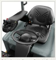
Fully adjustable Operator Restraint System (ORS) with side-wings and lumbar support.
