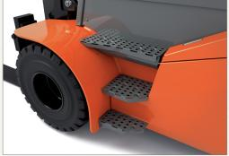
Large entry window with wide steps and double driver assist grips ensure fatigue is minimized in applications that require repeatedly getting in and out.
